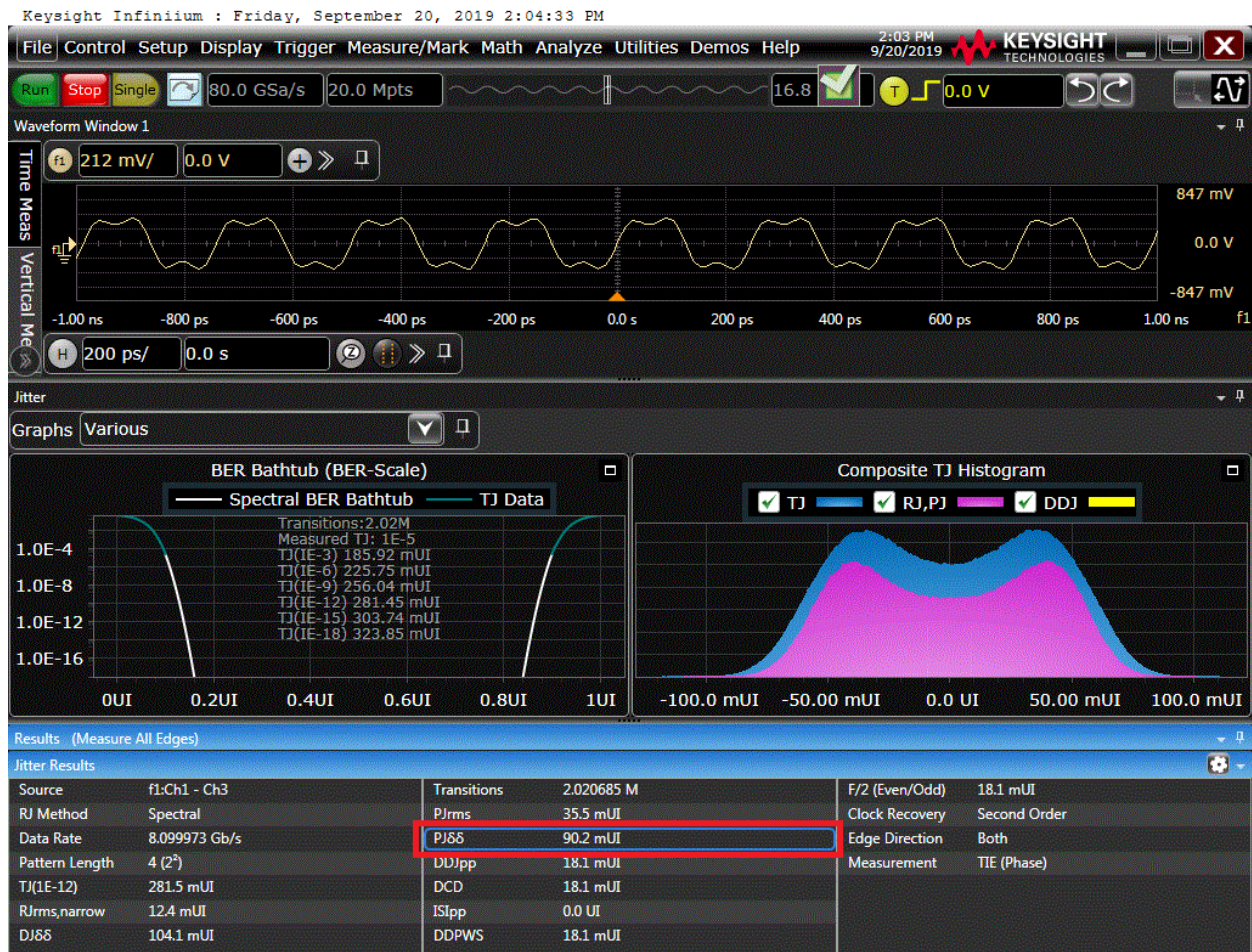
FIGURE 62. HBR3 SJ_{\text{FIXED}} MEASUREMENT EXAMPLE ON KEYSIGHT SCOPE (NOT SHOWING TARGET 80mUI)
