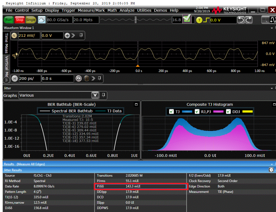
FIGURE 66. HBR3 SJ SWEEP MEASUREMENT EXAMPLE ON KEYSIGHT SCOPE
