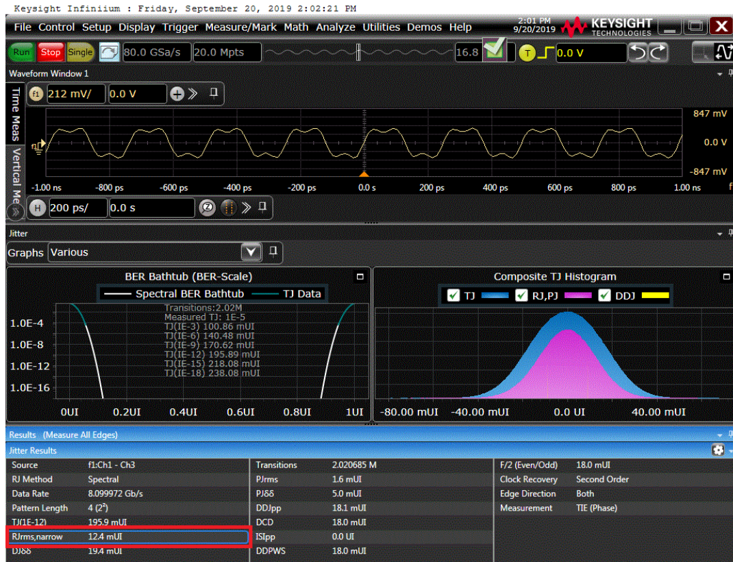
FIGURE 58. HBR3 RJ MEASUREMENT EXAMPLE ON KEYSIGHT SCOPE
