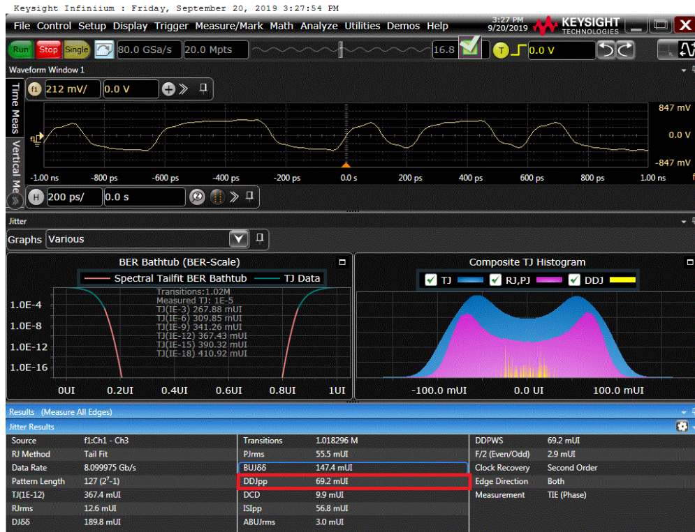
FIGURE 69. HBR3 ISI MEASUREMENT EXAMPLE ON KEYSIGHT SCOPE
