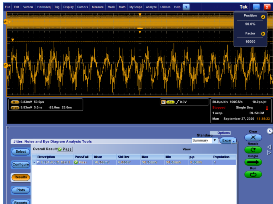
FIGURE 76. CALIBRATION TO PHASE MATCH ON TEKTRONIX SCOPE
