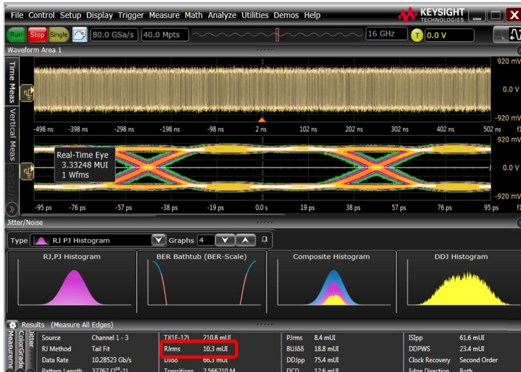
FIGURE 89. CALIBRATE RJ AMPLITUDE #2 ON KEYSIGHT SCOPE
