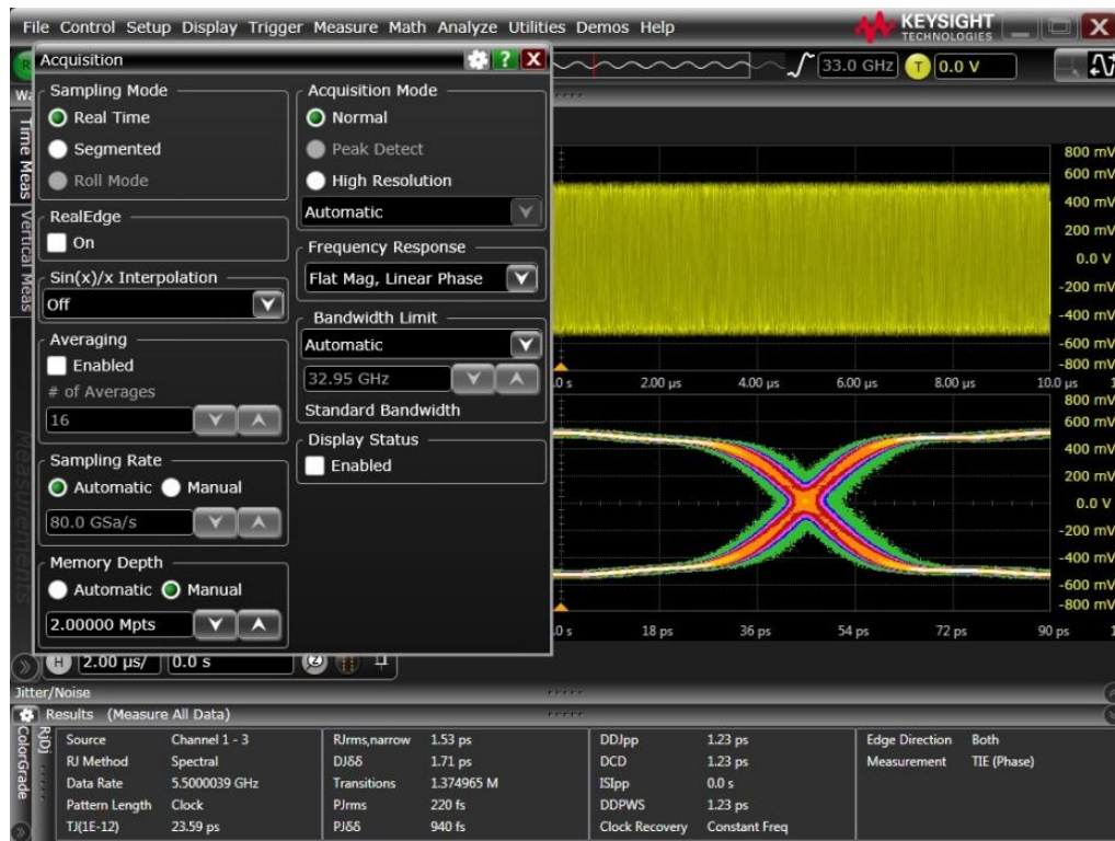
FIGURE 76. OSCILLOSCOPE VERTICAL AND HORIZONTAL SETUP
