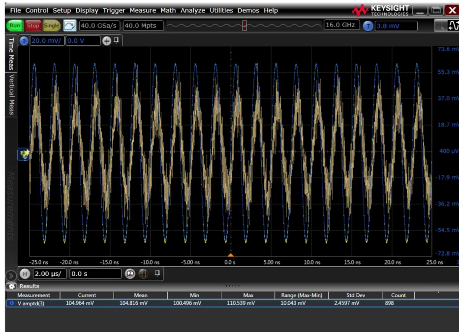
FIGURE 83. CALIBRATION TO PHASE MATCH ON KEYSIGHT SCOPE
