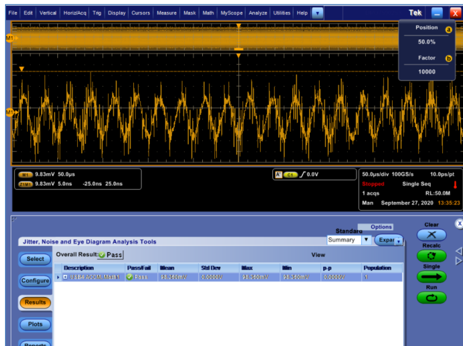
FIGURE 84. CALIBRATION TO PHASE MATCH ON TEKTRONIX SCOPE
