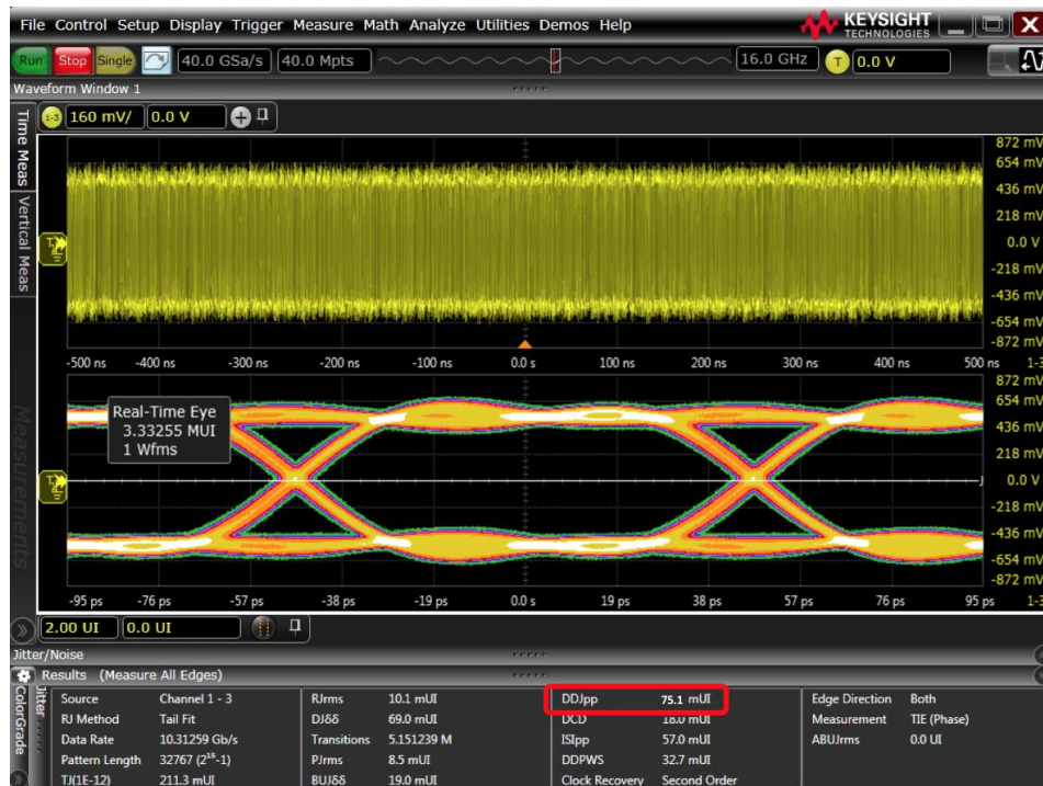
FIGURE 81. OPTIMIZED PRESET (MINIMUM DDJPP) MEASUREMENT ON KEYSIGHT SCOPE
