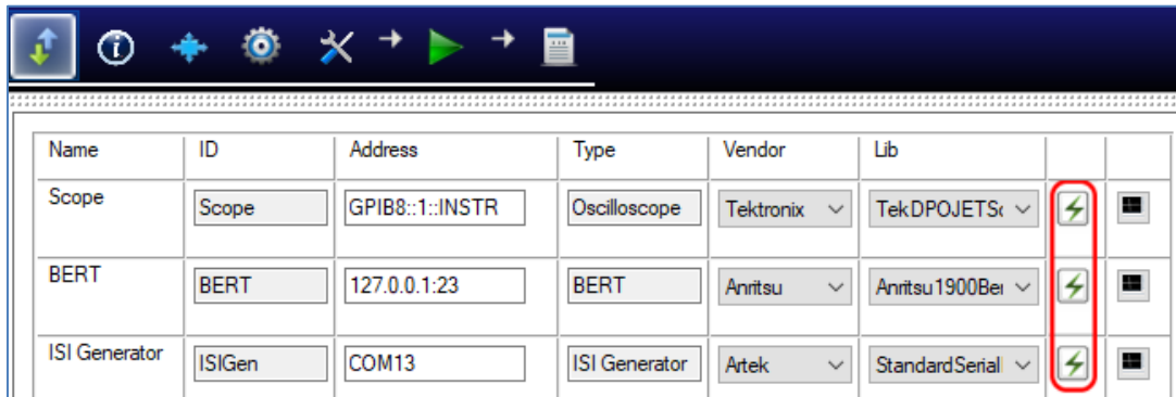
FIGURE 5. CONNECT INSTRUMENTS WITH GRL SOFTWARE
