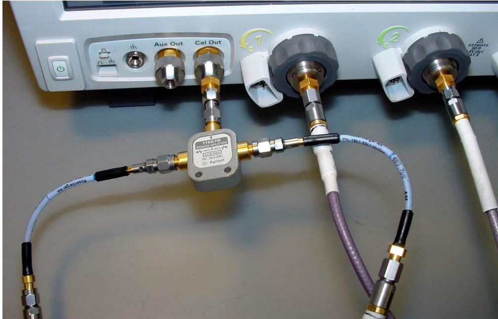
FIGURE 74. SCOPE DESKEW SETUP
