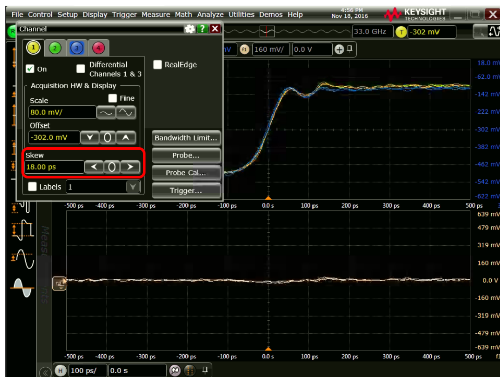
FIGURE 80. SCOPE DE-SKEW PROCESS – ADJUST SKEW
