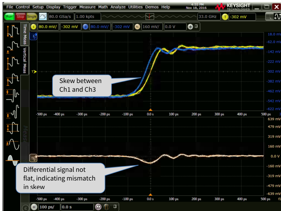
FIGURE 77. SCOPE DE-SKEW OSCILLOSCOPE DISPLAY
