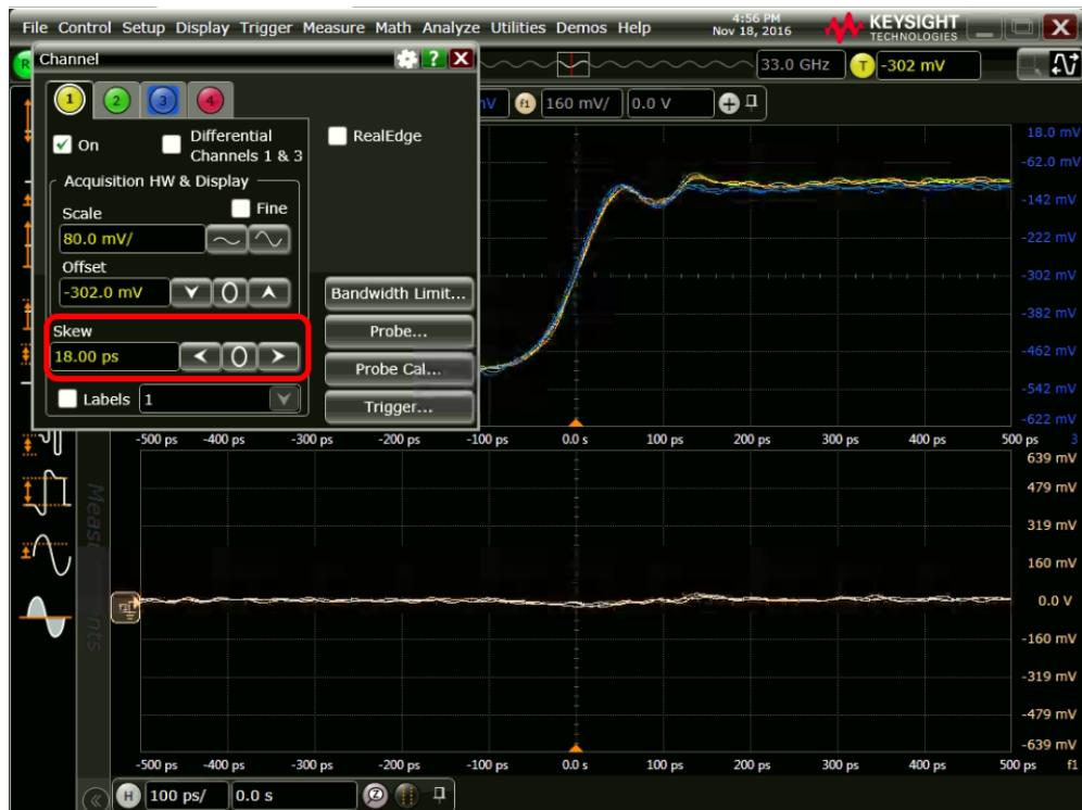
FIGURE 80. SCOPE DE-SKEW PROCESS – ADJUST SKEW
