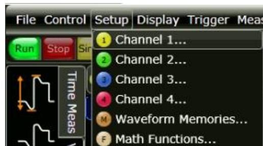
FIGURE 79. SCOPE DE-SKEW PROCESS – OPEN CHANNEL WINDOW
