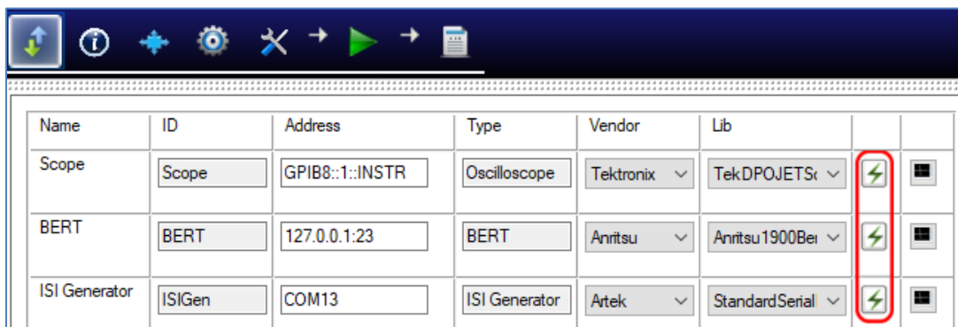
FIGURE 5. CONNECT INSTRUMENTS WITH GRL-PXE4-BASE-RXA SOFTWARE
