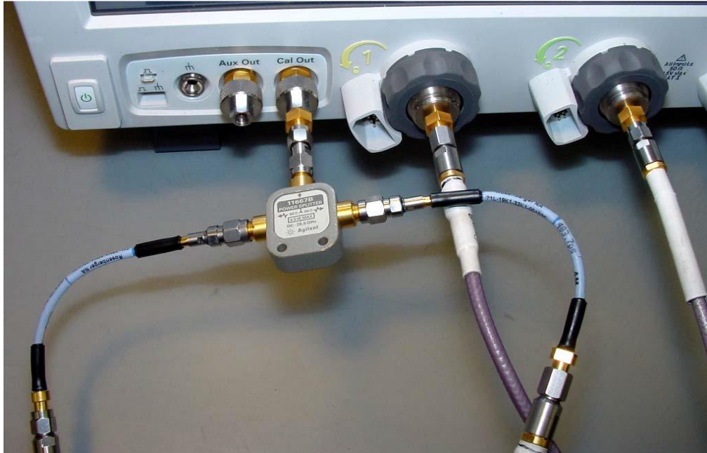
FIGURE 74. SCOPE DESKEW SETUP
