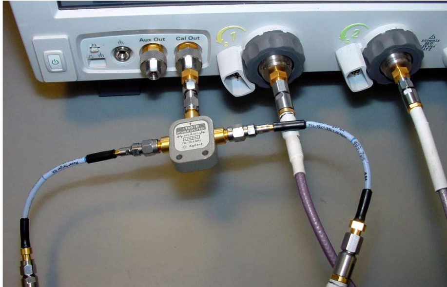
FIGURE 59. SCOPE DESKEW SETUP
