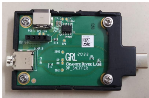
FIGURE 3.6: CLOSE-UP OF GRL-C2-DP-AUX-SNIF BOARD TEST FIXTURE
