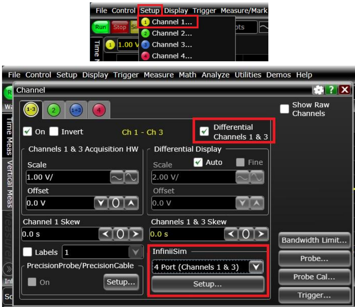
FIGURE 85. SMA CABLE TRANSFER FUNCTION– SET UP SCOPE CHANNELS 1 & 3
