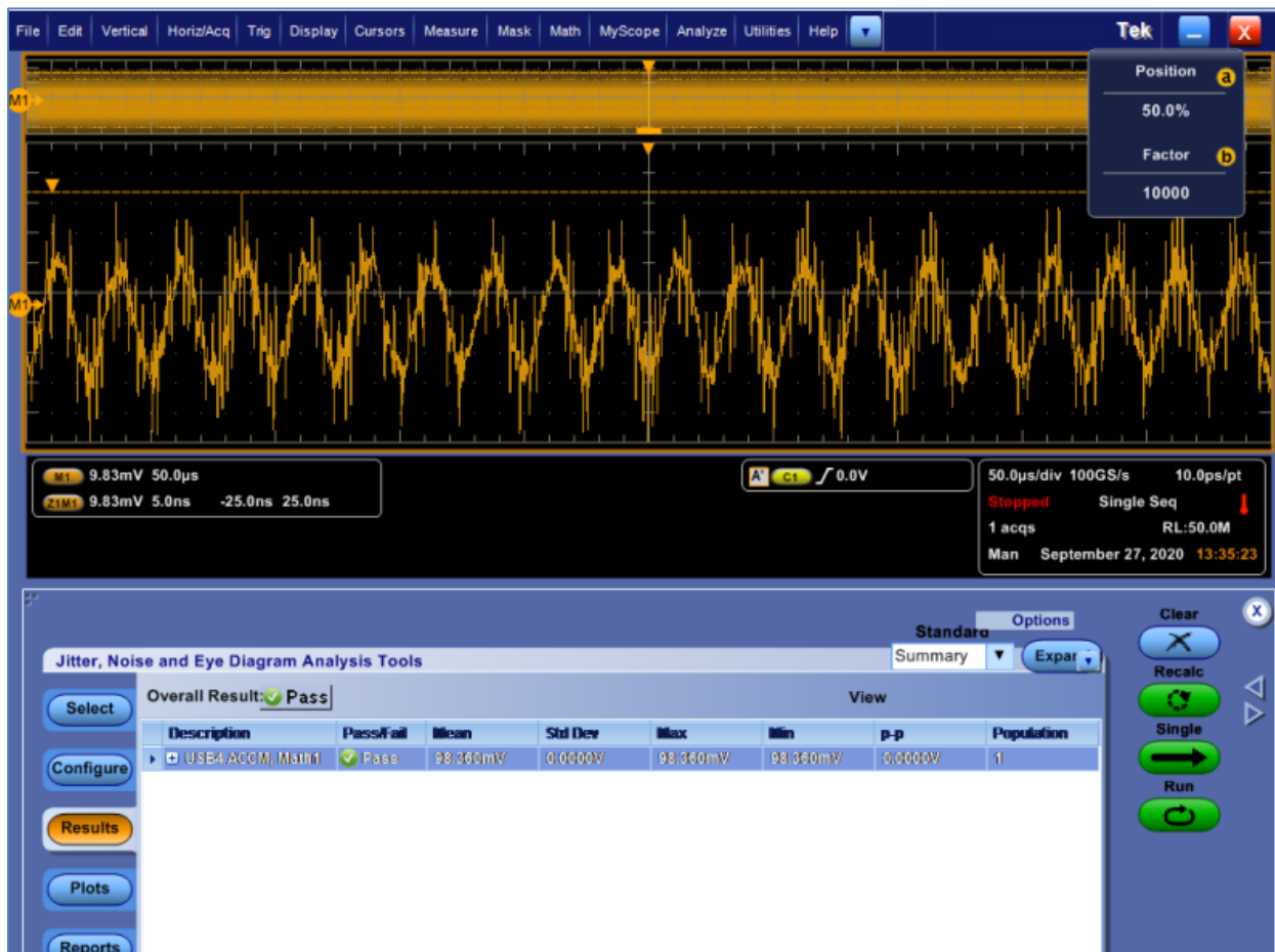
FIGURE 56. CALIBRATION TO PHASE MATCH ON TEKTRONIX SCOPE
