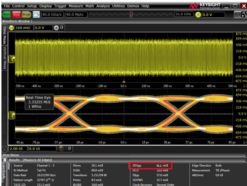
FIGURE 53. OPTIMIZED PRESET (MINIMUM DDJPP) MEASUREMENT ON KEYSIGHT SCOPE
