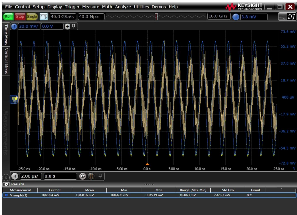
FIGURE 55. CALIBRATION TO PHASE MATCH ON KEYSIGHT SCOPE
