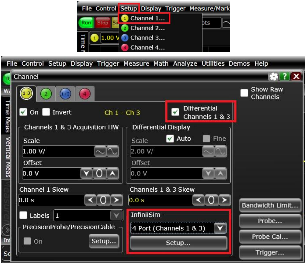
FIGURE 57. SMA CABLE TRANSFER FUNCTION– SET UP SCOPE CHANNELS 1 & 3
