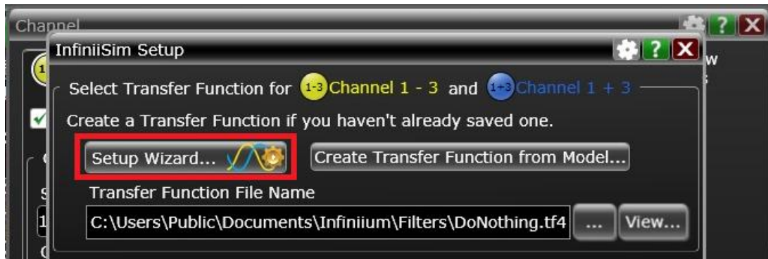
FIGURE 58. SMA CABLE TRANSFER FUNCTION– SELECT SETUP WIZARD ON SCOPE
