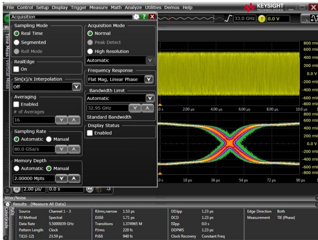
FIGURE 64. OSCILLOSCOPE VERTICAL AND HORIZONTAL SETUP
