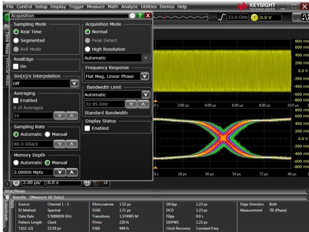
FIGURE 75. OSCILLOSCOPE VERTICAL AND HORIZONTAL SETUP
