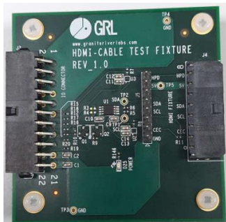
GRL-HDMI Cable Test Fixture – Connects to the Expansion IO connector at the rear of the NOVA-S03 analyzer hardware through the HDMI-IO-Cable. The user can connect the low-speed lines coming from the other end of the GRL-HDMI Cable Test Fixture to the HDMI port in front of the NOVA-S03 analyzer hardware through jumper wires.
